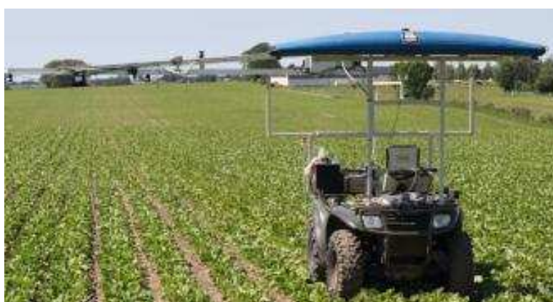
Figure 2.4 In 2011-2013, an ATV equipped with sensors from Skye and Yara was used to measure canopy reflectance.
